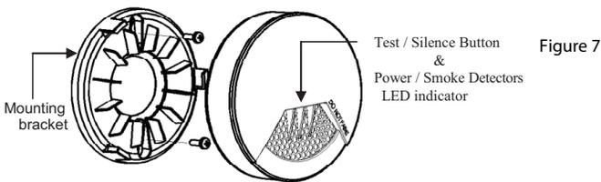
**CAUTION:** This smoke detector comes with cover latches that will prevent the smoke detector cover from closing if battery is not installed. This tells you that the detector will not work until a new battery is properly installed.
